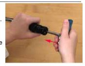
Insert the Locking Key into the jam nut by sliding it forward on the CART Tool. Only finger pressure will be needed to tell when the Locking Key meets the jam nut. It may be necessary to slightly rotate the Locking Key to allow the hex on the key to engage the hex on the nut. When the engagement occurs, you will feel the Locking Key slide further forward
