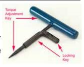
The outer key is the Locking Key. It is "L" shaped and has a larger hex size. This key engages a jam nut inside the wrench to lock the torque setting in place. To adjust the torque, the nuts must first be disengaged from contact with each other.
