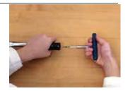
Insert the Torque Adjustment Key into the wrench as shown. The Locking Key should not yet be engaged. The Torque Adjustment Key will slide easily into the center of the wrench adjustment mechanism. Some slight rotation of the key may be necessary to assure it fully engages the torque adjustment mechanism.
