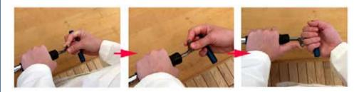
Grasp the wrench and the CART Tool. Hold the Adjustment Key in place and rotate the Locking Key clockwise until it jams against the torque adjustment mechanism. This will be felt as firm resistance to further rotation. Then hold the Locking Key in place and attempt to rotate the Adjustment Key counterclockwise. It should not move more than a small fraction of a turn. When that is the case, the torque is set and locked in place.
