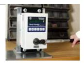
Cycle ("click") the torque wrench 4 times to determine the current torque setting. Read and note the last reading displayed by the tester.
